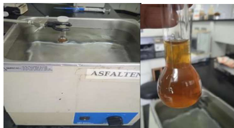
Fig. 5. Ultrasound to solubilize the lignin mixture obtained (LO) with NaOH 4%.
