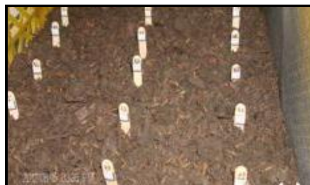
Fig.2. Experimental setup for preliminary biodegradation studies in composting soil.
